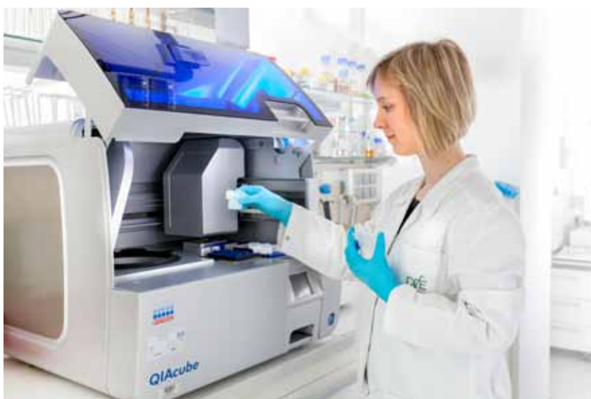
Figure 3: The QIAcube enables automated extraction of bacterial DNA from fecal samples of adults and infants. Later on, the DNA can be used to analyze the microbial composition in the gut.
