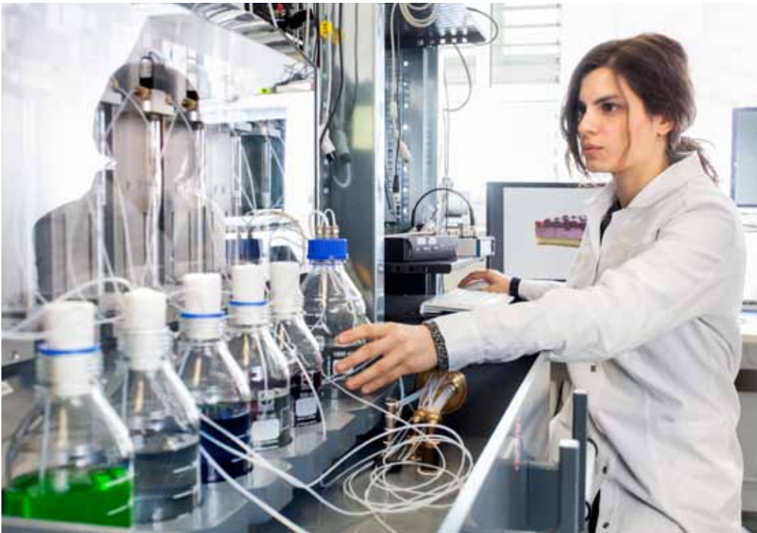
Figure 3: Exterior view of the computer-supported gustometer for testing taste perception. This high-precision device dispenses different amounts of solutions for taste tests.
