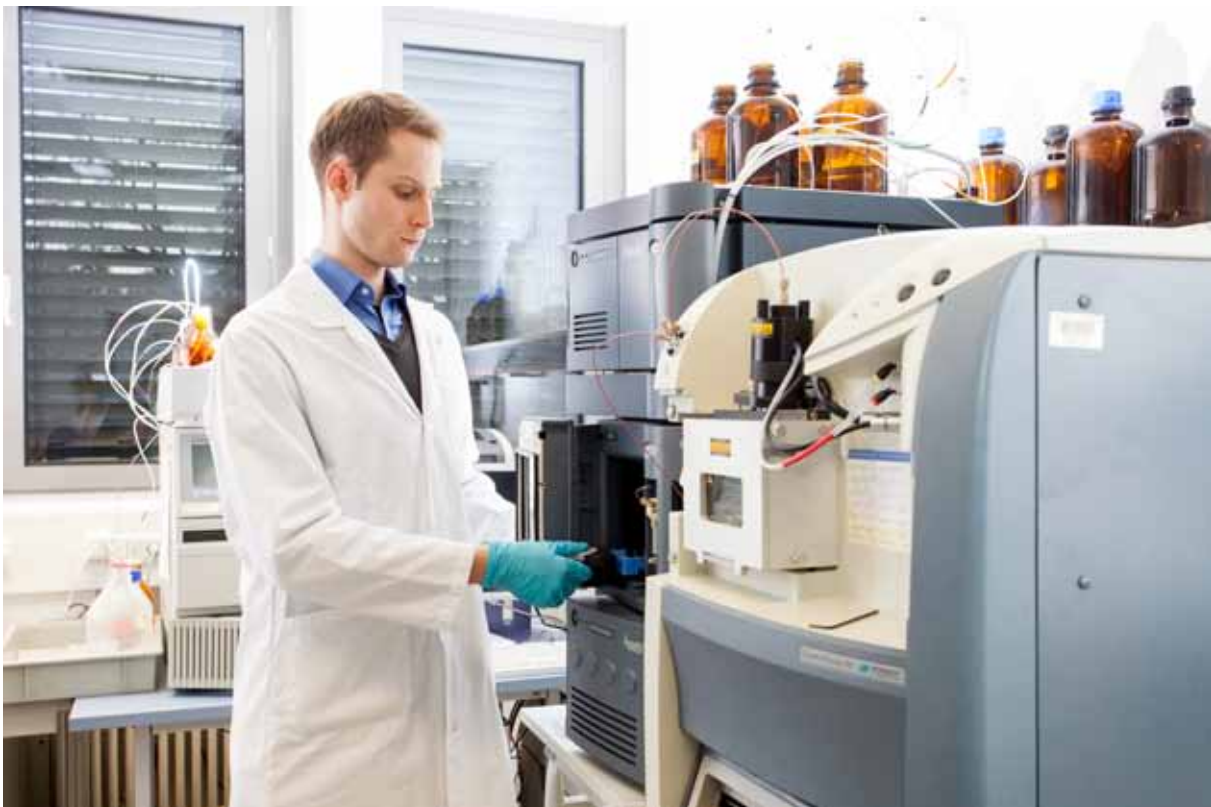
Figure 2: Scientist applying samples for the UPLC (Ultra Performance Liquid Chromatography) that is coupled to a mass spectrometer (foreground).
