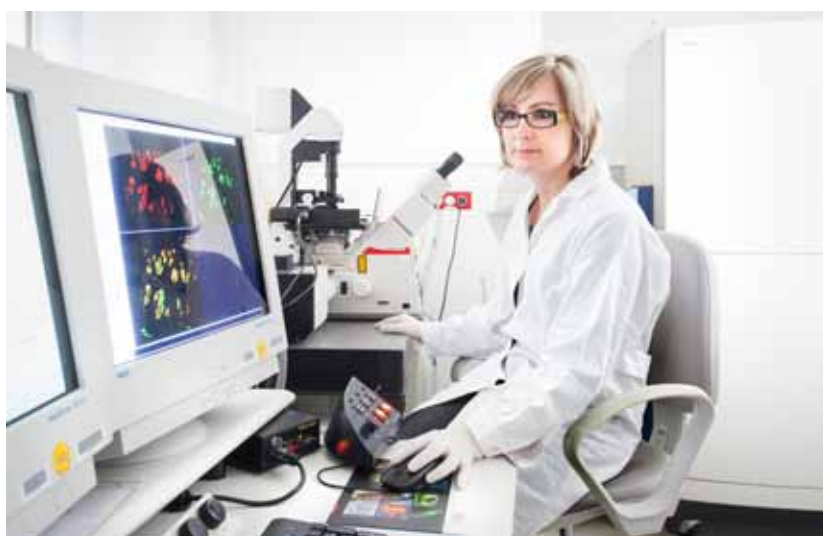
Figure 3: Technician of the department analyzes tissue samples using a confocal microscope. Confocal microscopy enables the observation of a stack of thin independent layers of the investigated sample ("optical slicing"), and thus of the distributions of different proteins within (intra)cellular structures.
