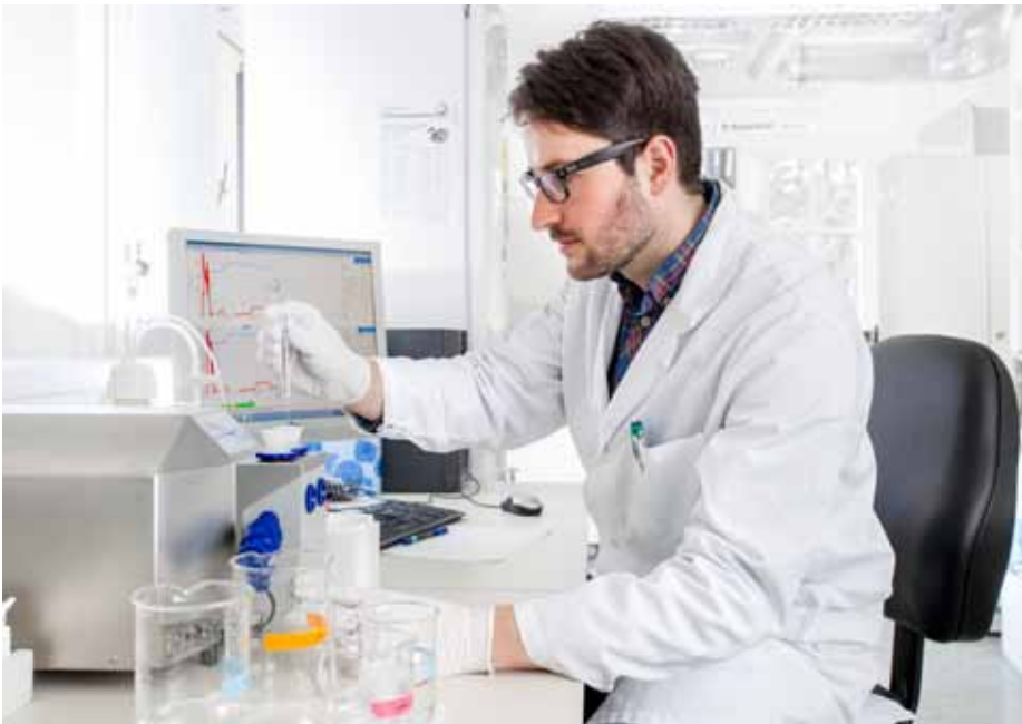
Figure 1: Scientist using high-resolution respirometry for analysis of mitochondrial function in biopsy samples of muscle, liver, and adipose tissue.
